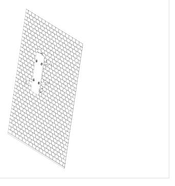
**Step2**: Align the rear notch of charger into the wall-mounted bracket and fit the screw holes of the right and left side.
